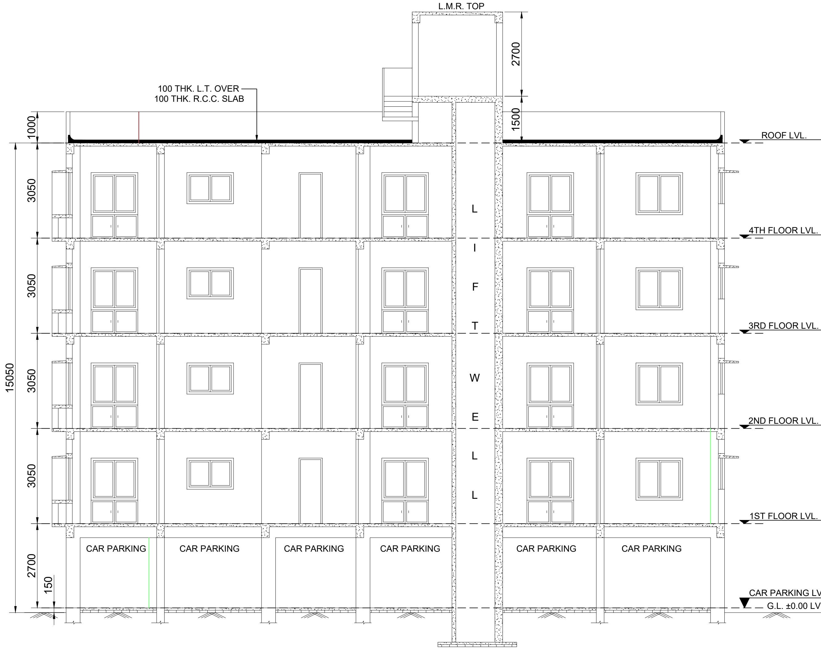
SECTION - Y-Y1 SCALE - 1:100
